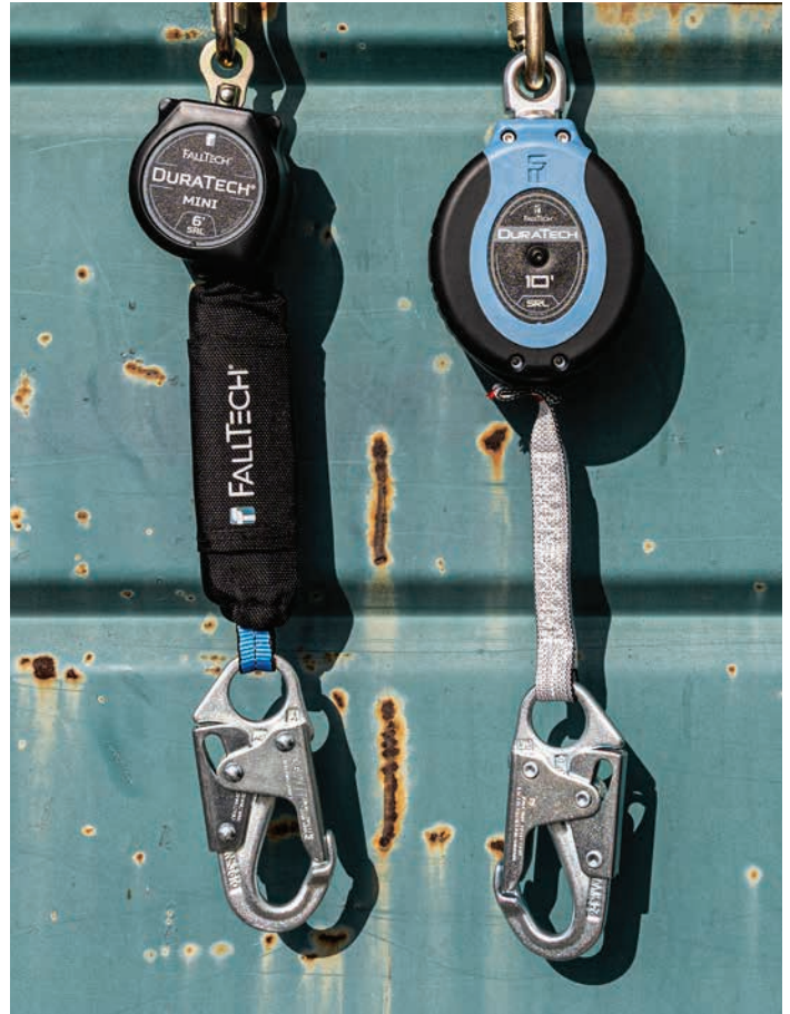
Two Class 1 SRLs: external absorber (left) vs. internal brake (right). Note the size difference—internal brakes require more components and lifeline.
